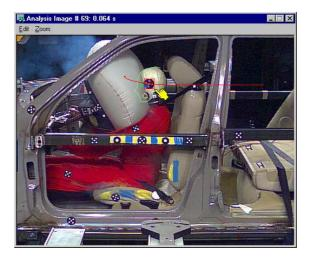
The FalCon **MovXact** module allows you to precisely analyze image sequences with the methods of 2D image measurement technology.
